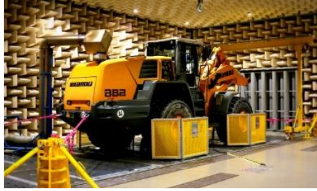
Acoustic all-wheel drive roller test bench
