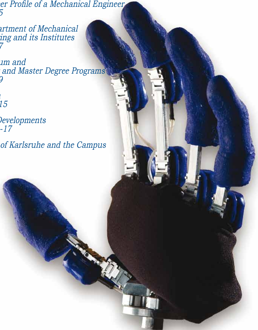
Fluidic robot hand of the Collaborative Research Center 588 'Humanoid Robots', Institute of Applied Computer Science/Automation
