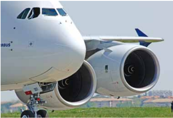
The AirBUS A380 is equipped with the Rolls Royce Trent 900 turbine engine. Institute of Thermal Turbomachinery
