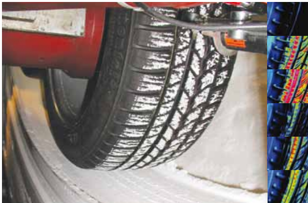
Transient temperature distribution on the surface of a rotating tire. Measurements are made by an internal drum test bench, the first of its kind in the world, designed for laboratory snow experiments at the Institute of Vehicle System Technology.
