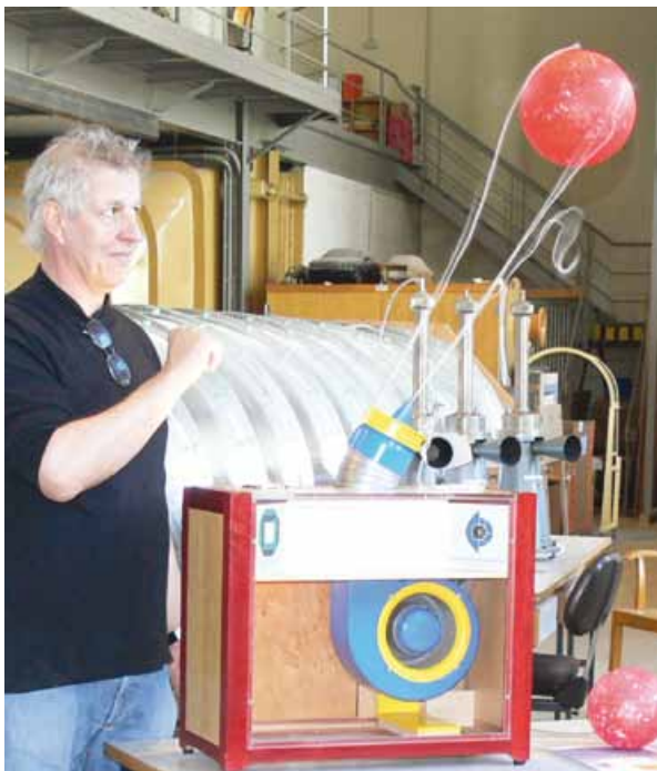
Demonstration of aerodynamic forces strong enough to allow a ball to hover. Department of Fluid Machinery
