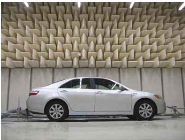
Comfort analysis of modern hybrid electric vehicles (HEVs) concerning vibration and acoustics (noise/vibration/harshness - NVH). Institute of Product Development
