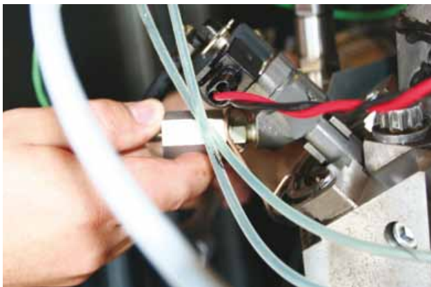
Single cylinder engine for fuel injection experiments in a specially adapted detached cylinder head. A second injector has been attached at the side of the main injector. Institute of Internal Combustion Engines
